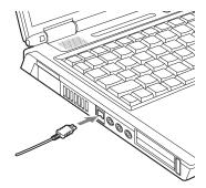
Figure 4-20. Connecting an IEEE 1394 Device
